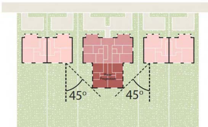
Figure 2.11b: Depth of projection no greater than 45 degrees as measured from the middle of the window of the closest ground floor habitable room on the rear wall of the main neighbouring property on both sides.
